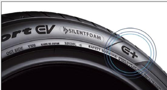
motor, a level of quietness suitable for silent-running electric vehicles, and improved power and energy consumption efficiency to extend cruising range. We have introduced our own unique E+ mark to indicate that a passenger car, bus, or truck tyre is suitable for EV use, and will apply this to products going forward. By displaying the E+ mark, we clearly indicate to customers which products are compatible with electric vehicles so that they are able to choose the right tyre.
