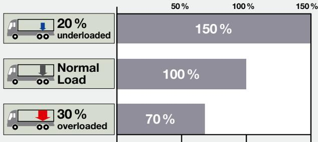
Tyre wear depends upon the load carried. YOKOHAMA recommends maintaining the correct axle and payloads.
