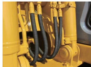
High-pressure hoses featured in construction machinery
